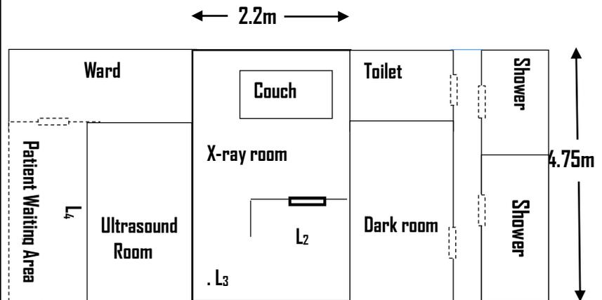
Wall thickness of X-ray/imaging room-26cm.
